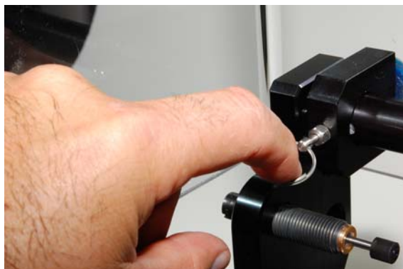
Pull ring or if equipped the small knob back to release the cover.
